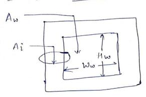
As the iron Area of the leg Ai and the window area Aw = (height of the window Hwx width of the window Hwx width of the window Ww) increases the Size of the transformer also Increases. The Size of the transformer Increases as the output of the transformer Increases.
